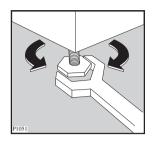
Any necessary adjustment can be made with a spanner. Accurate levelling prevents vibration, noise and displacement of the machine during operation. Some vibration is inevitable, especially if mounted on a wooden floor.
